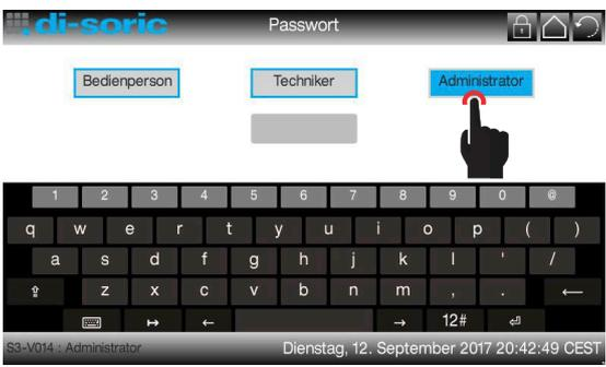
This system supports three user roles, two of which (Administrator and Technician) can be protected by a password. If a password has been issued, it has to be entered using the onscreen keyboard. If no password has been issued, the corresponding main menu is called up immediately by tapping the respective button.
