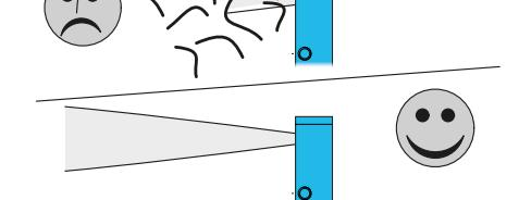
The transducer surface as well as the field of the detection beam must be kept free mandatorily. You need to pay attention on having no disturbing objects between the sensor and the target object within the detection beam.
