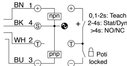
IRSD-50P-G3-B4 inductive ring sensor with potentiometer
