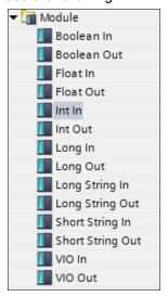
You must manually drag and drop "Boolean In\_1" and "Float In\_1" into the Device Overview pane. Click on "Boolean In\_1", and TIA will highlight the slot to drag it to. Repeat this for "Float In\_1". TIA will only allow you to insert them into their proper slot position.
