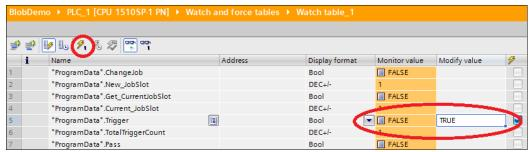
You will see the **InstancePoints**, **Status**, and **RadiusDatum** change based on the picture. The pass and fail bools will indicate whether the inspection has passed or failed. Also, the appropriate counters will have incremented. Each click of the lightning bolt button will cause an inspection which will bounce from one image to the next. One will pass and the next will fail.
