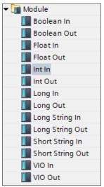
You must manually drag and drop "Int In" into the Device Overview pane. Click "Int In" and TIA will highlight the slot to drag it to. TIA will only allow you to insert them into their proper slot position.
