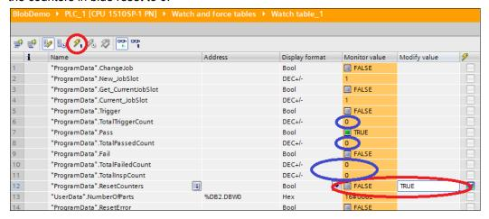
If you clear this again, set the Trigger to TRUE, and click the lightning bolt button again, you will notice that the counts start at 1 on both the PLC counters and CS50 Software counters.
