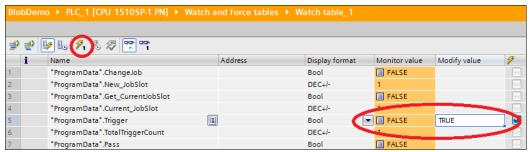
You will see the **NumberOfParts** change to either **2** or **5**. The pass and fail bools will indicate whether the inspection has passed or failed. Also, the appropriate counters will have incremented. Each click of the lightning bolt button will cause an inspection, which will bounce from one image to the next. One will pass and the next will fail.
