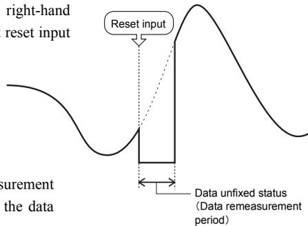
The table below shows the measurement value display and output under the data unfixed status or alarm status.
