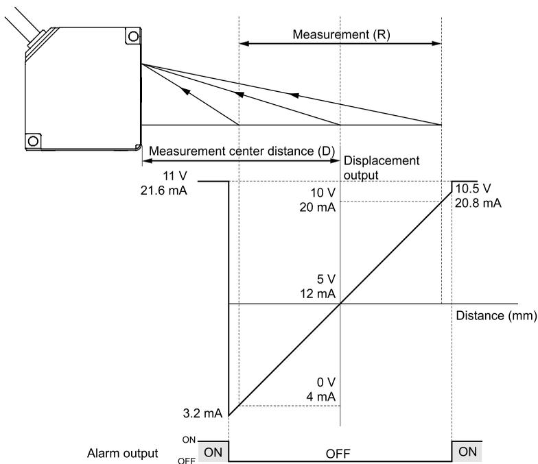
\*1 In the figure above, analog output setting is used as the initial setting.
